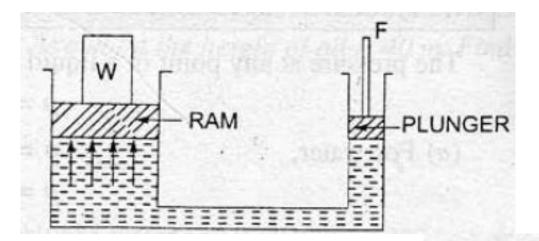
Due to Pascal's law, the intensity of pressure will be equally transmitted in all directions. Hence the pressure intensity at the ram
