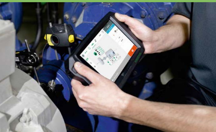
Laser technology is one of the most precise methods for correctly aligning rotating shafts.
