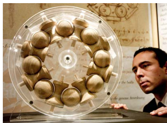
Even long before the birth of Christ, rolling logs were used to reduce friction, like the Egyptians did for building pyramids as shown here. Universal genius Leonardo da Vinci is regarded as the inventor of the ball bearing. Depicted above is a replica based on original drawings.
